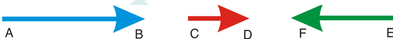
Fig. 01 – All three vectors share the same direction but differ in magnitude: AB > EF > CD . Blue and red vectors have the same sense; the green vector has the opposite sense.
